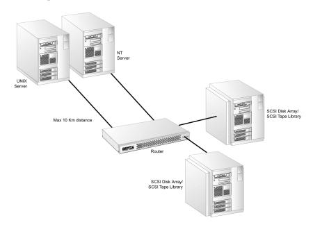
Figure 2-7. Multiple server configuration example
